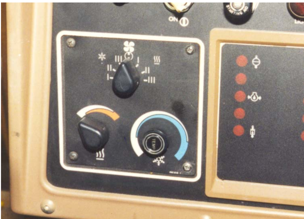
Thermostat in location on dash control panel.
