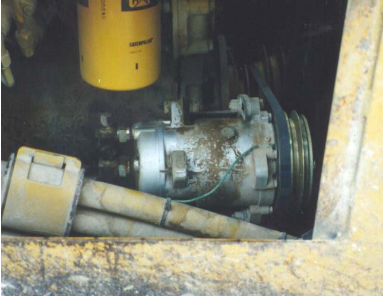
Compressor mounted in place - new style compressor.
