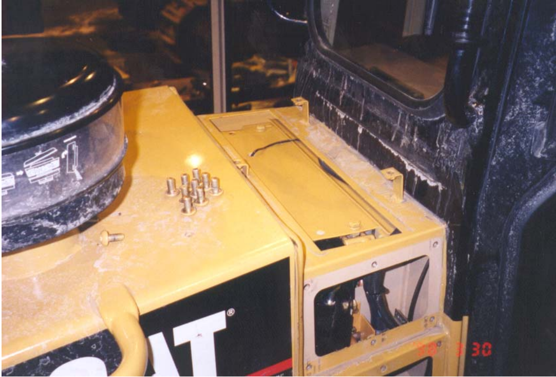
Evaporator cover in place with thermostat.
